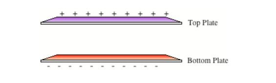
Note that the electric field strength in the **interior** region between two oppositely charged parallel plates is **constant**; the field is <u>not</u> stronger as you get closer to either plate.
