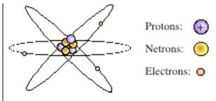
An electron stores the smallest individual unit of charge,  $\mathbf{q} = 1.6 \times 10^{-19}$  C. The total charge on an object is calculated using the formula Q = nq, where Q represents the total charge and *n* represents the number of electrons. All electrical charges are due to an \_\_\_\_\_\_ or \_\_\_\_\_ of electrons.
