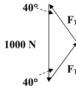
In this case both sides  $F_T$  are equal because we have an isosceles triangle. As well, by examining the vector triangle, we are given one side and the two included angles and asked to find one of the other sides. Therefore, use the Sine Law to solve (check formula sheet for reference):
