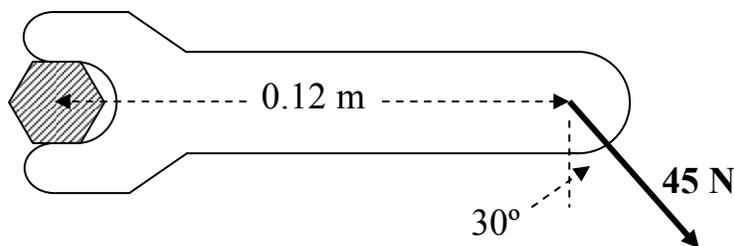
The wrench will turn, but with a reduced torque. To determine the magnitude of this torque, components of the force vector must be taken that are parallel and perpendicular to the distance from the pivot:
