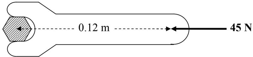
Clearly, the wrench won't turn in this case (though it might break if the force is large enough). In other words, no torque will happen in this arrangement.
