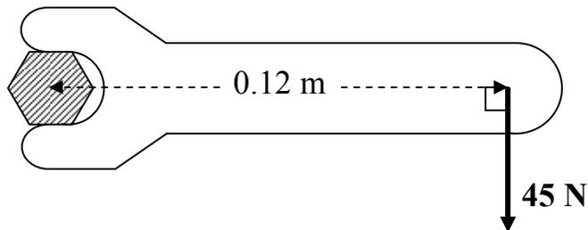
The torque here is calculated to be  $\tau = 45(0.12) = 5.4 \text{ N-m}$ , in a *clockwise* direction. Note the following:
