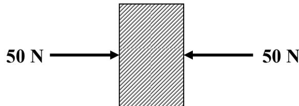
To be more specific, if the line of action of each force acting on the body passes through a common point, the forces are termed *concurrent*. This is true regardless of how many forces act on the body.
