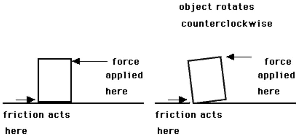
In the example above, the applied force produces a counter-clockwise torque about the lower-left corner pivot, while the centre-of-gravity of the object creates a clockwise torque about the same pivot. If the applied force is large enough, or high enough up from the pivot, the object will rotate in a counterclockwise direction, pivoting around its lower-left corner.
