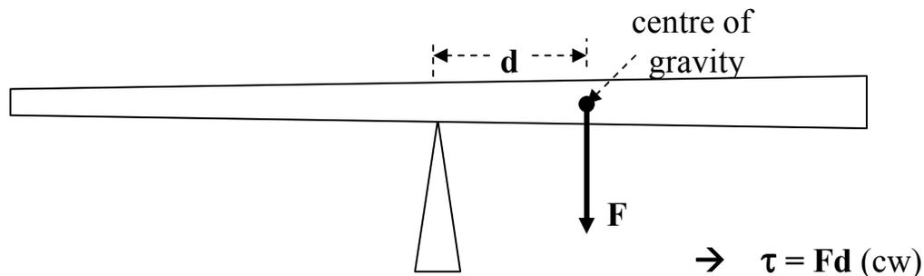
**Example #9:** Calculate the net torque acting in the system below. Note that the beam is uniform, has a mass of 0.85 kg, and a length of 6.2 m.
