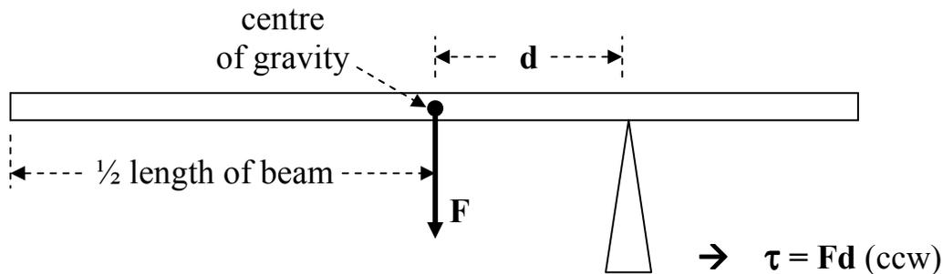
For a non-uniform beam (centre of gravity must be indicated in the question):
