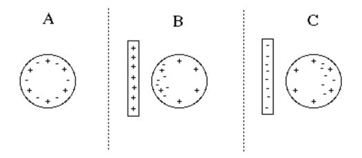
An electroscope is a simple device that detects static charges. Importantly, an electroscope can show the effects of charging by both conduction and induction.
