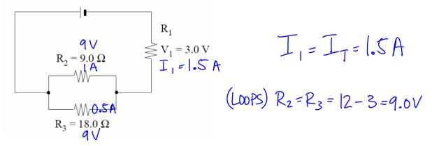
36. What is the total power dissipated in the three resistors below?
