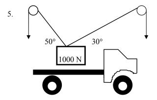
What must the tension in each cable be in the diagram in order to support the cargo in static equilibrium? Note that pulleys only change the *direction* of the force, not the magnitude. 6. What will the unknown angle  $\theta$  be in order for the pulley system to the right to be in static equilibrium? Note that the 80 N weight is attached to a free-moving pulley, and the cable is fastened to the wall on the left.
