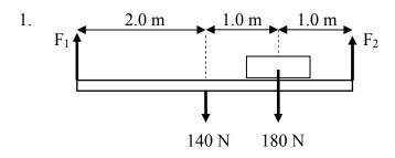
For the left diagram, what upward force  $F_2$  is required to keep the beam in both static and rotational equilibrium?
