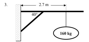
Examine the diagram to the left. If the horizontal uniform 3.6 m-long beam has a mass of 82 kg, and the location of the support beam is 1.4 m from the wall, what force is the support beam supplying to keep the system in equilibrium?
