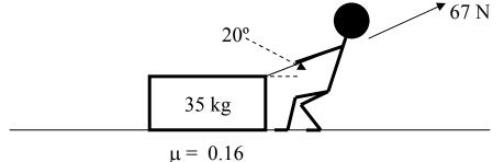
Start with a f.b. diagram, and break the applied force of 67 N into components: (note that vectors are <u>not</u> drawn to scale)
