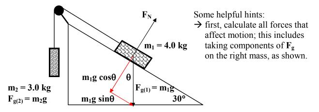
→Next step: to find the acceleration, consider the *whole system*. Note which force is greater; that will be the direction of the net force and the acceleration.
