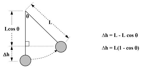
Example #14: A pendulum bob of mass 5.0 kg falls through a height of 25 cm as it swings from maximum height to lowest position.
