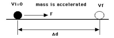
Note that kinetic energy changes as the speed of the object changes. The work done against inertia to accelerate the mass a distance  $\mathbf{d}$  can be determined <u>*two*</u> ways:
