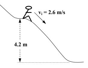
a) at start,  $E_{+} = E_{p} + E_{k}$  $= 60(9.8)(4.2) + \frac{1}{2}(60)(2.6)^{2}$ = 2672.4.1 at bottom, Er = Ek  $Z_{672.4} = \pm (60) v^{2}$  $v = 9.4 \, m/s$ b) at botton: Er = Ek + heat  $2672.4 = \frac{1}{2}(60)(6)^2 + heat$ heat =  $1.6 \times 10^3$  J
