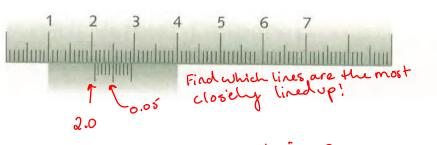
So... the measurement is 2.05 cm (2,0+0.05) MEASUREMENT UNIT Name:
