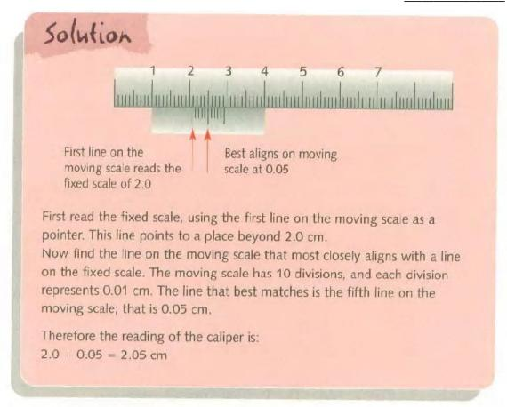
**Example #2:** Read the following Vernier caliper calibrated in metric units.
