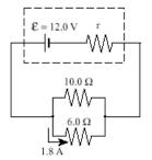
If the current through the 6.0  $\Omega$  resistor is 1.8 A , what is the internal resistance r ?
