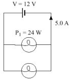
The power output of one of the bulbs is  $P_1 = 24$  W. What is the power output of the other bulb?
